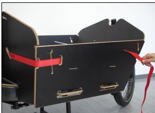
fig. 6: routing the tensioning belt
