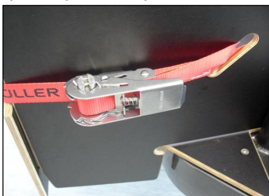
fig. 8: tightening the tensioning belt
